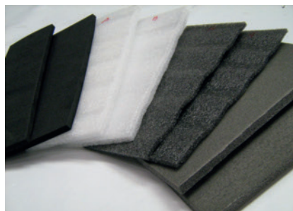
Fig. 1. Besides foams with different surfaces, multiwall panels can also be treated by the linear plasma process; where conventional corona treatment may not be used
