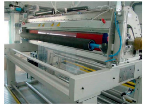
Fig. 4. The stations are designed for inline treatment and can treat, for example, web widths of 2 m at production speeds of 300 m/min
