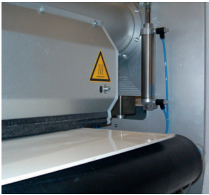
Fig. 2. This surface technology can be used to treat materials of any thickness; atmospheric pressure plasma modifies the surface on a sub nanometer scale
